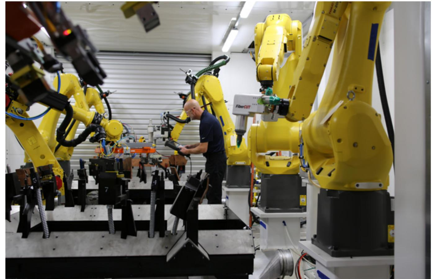
The Newton robotic laser cutting head is controlled directly from the robot teach pendant. Robot users can easily transition to the Newton head because the programming is familiar and easy to use.
