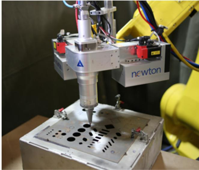
✓ The Newton head is a robot-mounted, 2-axis shape-cutting device that offers path accuracy up to  $\pm 0.05$  mm within a 30-mm operating range. The device is also capable of fast laser hole cutting speeds at 0.3 sec. for common size features.
