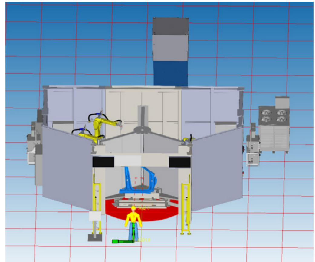
✓ A flexible robotic workcell manages material flow through a turntable axis, often referred to as an interchange axis. These types of robotic workcells provide the user with a balanced load and unload time within the laser processing cycle.
